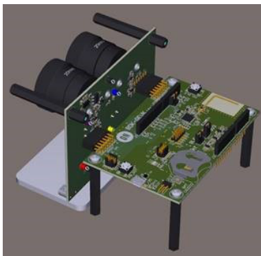
Figure 14. SiPM dToF LiDAR Reference Platform
