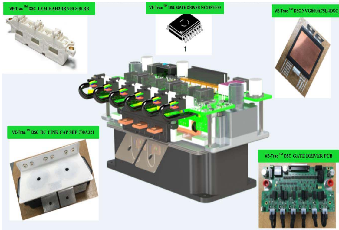
Figure 4. Major Components that Make Up the Evaluation Kit
