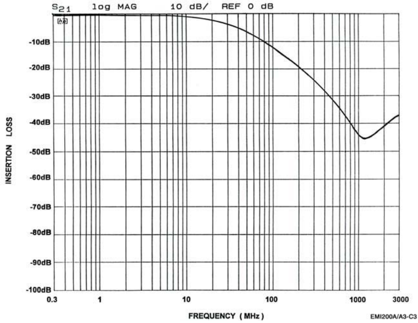
Figure 3. Speaker 1 Circuit (A3-C3) EMI Filter Performance
