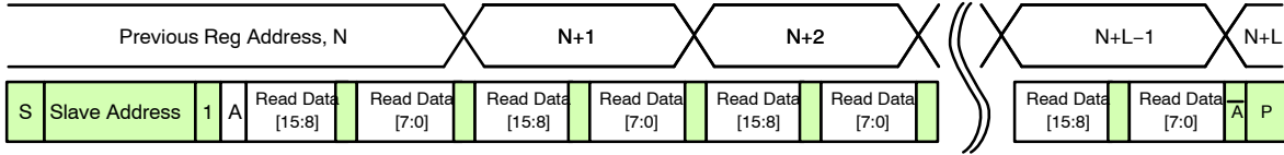
Figure 16. Sequential READ, Start from Current Location
