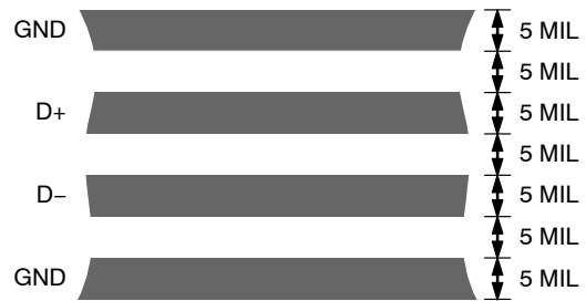
Figure 28. Arrangement of Signal Tracks
